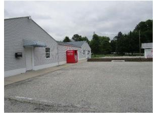
Parking in the front of the building can be converted into pervious pavement to capture and infiltrate stormwater runoff from the roof and parking lot. A preliminary soil assessment suggests that the soils have suitable drainage characteristics for green infrastructure.
