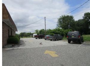
The section of parking spaces in the front of the building can be converted into pervious pavement to capture and infiltrate stormwater runoff from the roof and parking lot. A preliminary soil assessment suggests that the soils have suitable drainage characteristics for green infrastructure.
