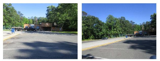
Parking spaces in front of the building can be converted into pervious pavement to allow the stormwater runoff from the road, roof, and parking lot to infiltrate the ground. The current conditions of the parking lot are poor; there are visible signs of erosion due to stormwater and cracking through the area. A preliminary soil assessment suggests that the soils have suitable drainage characteristics for green infrastructure.
