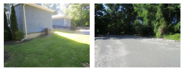
A rain garden can be installed in the turfgrass on the east side of the building to allow the stormwater runoff from the roof to infiltrate the ground. The strip of parking spaces on the far east side of the building can be converted into pervious pavement to capture and allow the stormwater from the roof and pavement to infiltrate into the ground. A preliminary soil assessment suggests that the soils have suitable drainage characteristics for green infrastructure.
