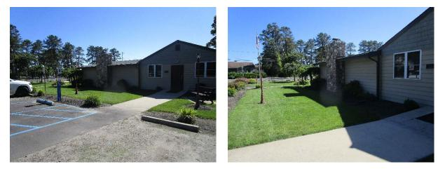
A rain garden can be installed at the east side of the building closest to the handicap parking spaces to allow stormwater runoff from the roof to infiltrate the ground and reduce the amount of runoff. A preliminary soil assessment suggests that the soils have suitable drainage characteristics for green infrastructure.
