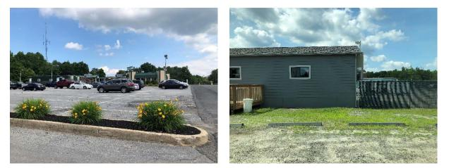
Rain gardens can be installed in turfgrass at the edges of the parking lots to capture, treat, and infiltrate stormwater runoff from the parking lots. A planter box can be installed on the shed in the back parking lot to provide an opportunity to beneficially reuse rooftop runoff as a demonstration project. A preliminary soil assessment suggests that more soil testing would be required before determining the soil's suitability for green infrastructure
