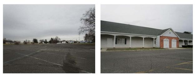
Parking spaces in the parking lot to the south of the building near the entrance can be converted to porous pavement to capture and infiltrate stormwater runoff from the parking lot. Two rain gardens can be installed at the back building's western entrance to capture and treat runoff from the roof. A preliminary soil assessment suggests that more soil testing would be required before determining the soil's suitability for green infrastructure.
