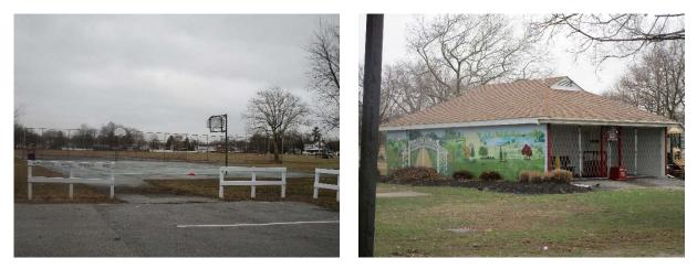
The basketball court can be replaced with porous asphalt which will also provide new asphalt for the basketball court. A rain garden can also be installed to the west of the parking lot to capture and treat stormwater runoff from the restroom building before it enters the catch basin. A preliminary soil assessment suggests that more soil testing would be required before determining the soil's suitability for green infrastructure.
