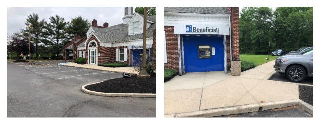
Parking spaces in front of the building's main entrance can be converted to porous pavement to capture and infiltrate stormwater runoff from the roof via the downspouts that convey water directly to the parking spaces. A rain garden can also be installed along the east side of the building by disconnecting downspouts from the building and redirecting the runoff into it. A preliminary soil assessment suggests that the soils have suitable drainage characteristics for green infrastructure.
