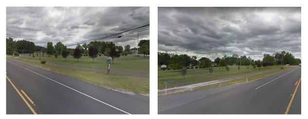
A bioswale can be installed in the right of way in the patch of grass between the road and sidewalk. The bioswale will catch runoff from the impervious road before entering a catch basin. This would convey stormwater in a controlled manner while also removing pollutants and allowing infiltration. A preliminary soil assessment suggests that the soils have suitable drainage characteristics for green infrastructure.
