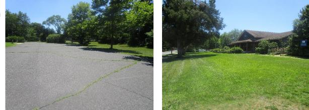
Bioretention systems can be installed in the turfgrass areas at each corner of the municipal building to capture runoff from the roof of the building as well as provide aesthetic value. Pervious pavement can be installed by replacing a section of the parking spaces near the edge of pavement to capture and infiltrate stormwater from the surrounding pavement. A preliminary soil assessment suggests that the soils have suitable drainage characteristics for green infrastructure.
