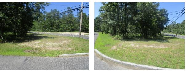
A bioretention system can be installed in the turfgrass area next to the intersection of Panama Road and County Road 563. The bioretention system will capture runoff from the impervious road and will allow infiltration of the runoff instead of runoff directly entering the nearby catch basin. A preliminary soil assessment suggests that the soils have suitable drainage characteristics for green infrastructure.
