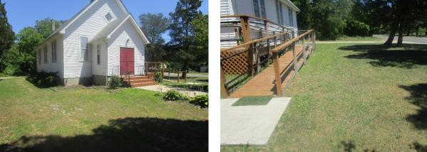
Bioretention systems can be installed next to the church in the turfgrass area on each side of the building. The bioretention systems can capture, treat, and infiltrate rooftop runoff. A preliminary soil assessment suggests that the soils have suitable drainage characteristics for green infrastructure.
