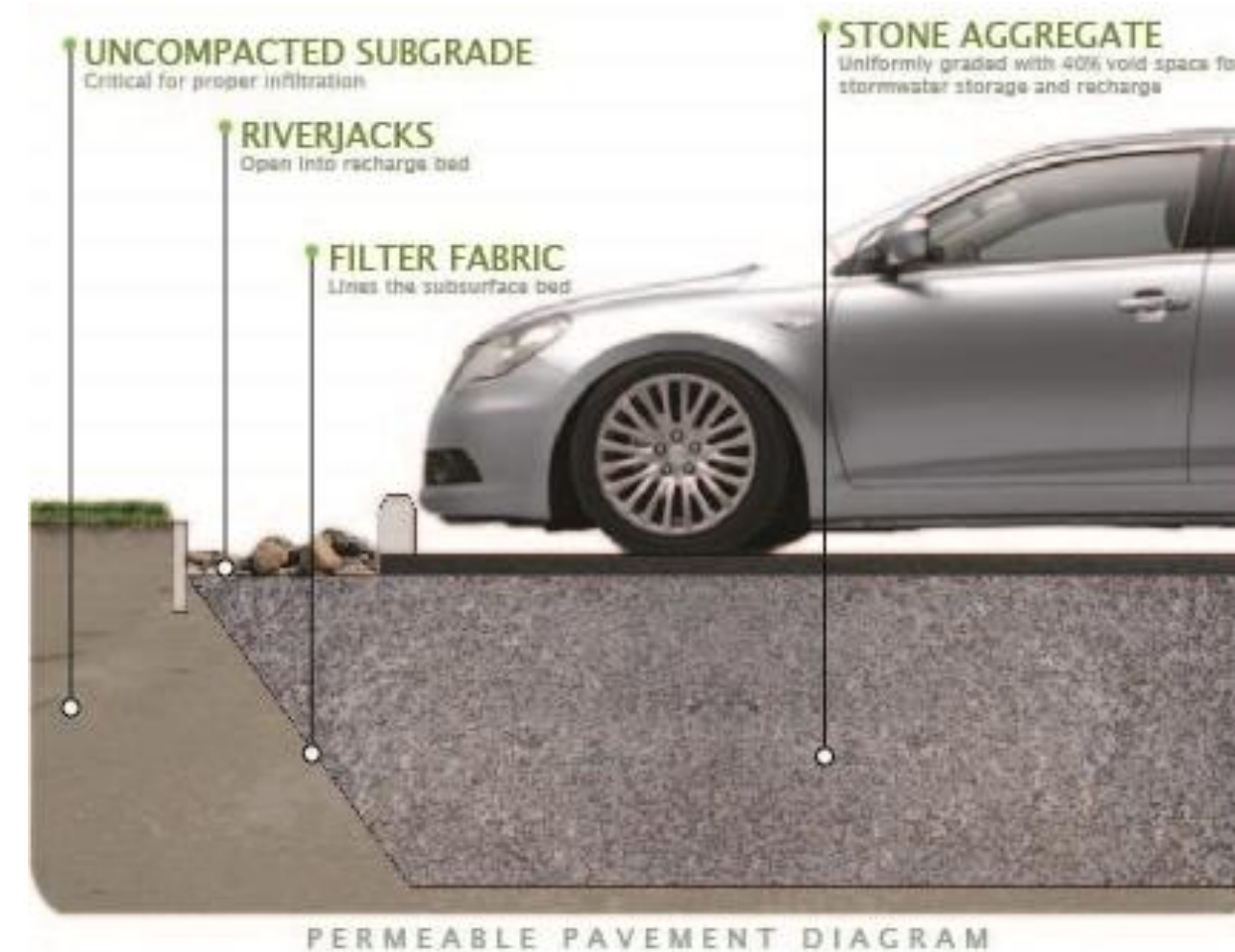
PERMEABLE PAVEMENT DIAGRAM
