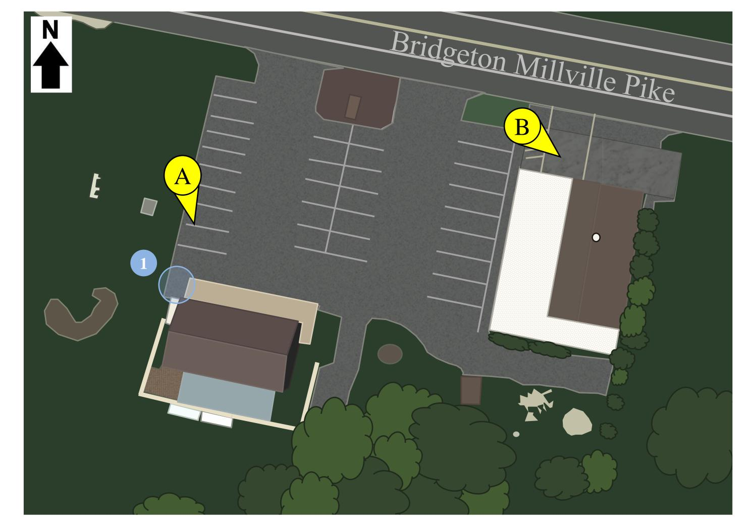
RAINWATER HARVESTING SYSTEM: Rainwater can be harvested from the roof of the west building and stored in a cistern on the northwest corner of the building. The water can then be used for watering gardens, washing vehicles, or for other non-potable uses.
