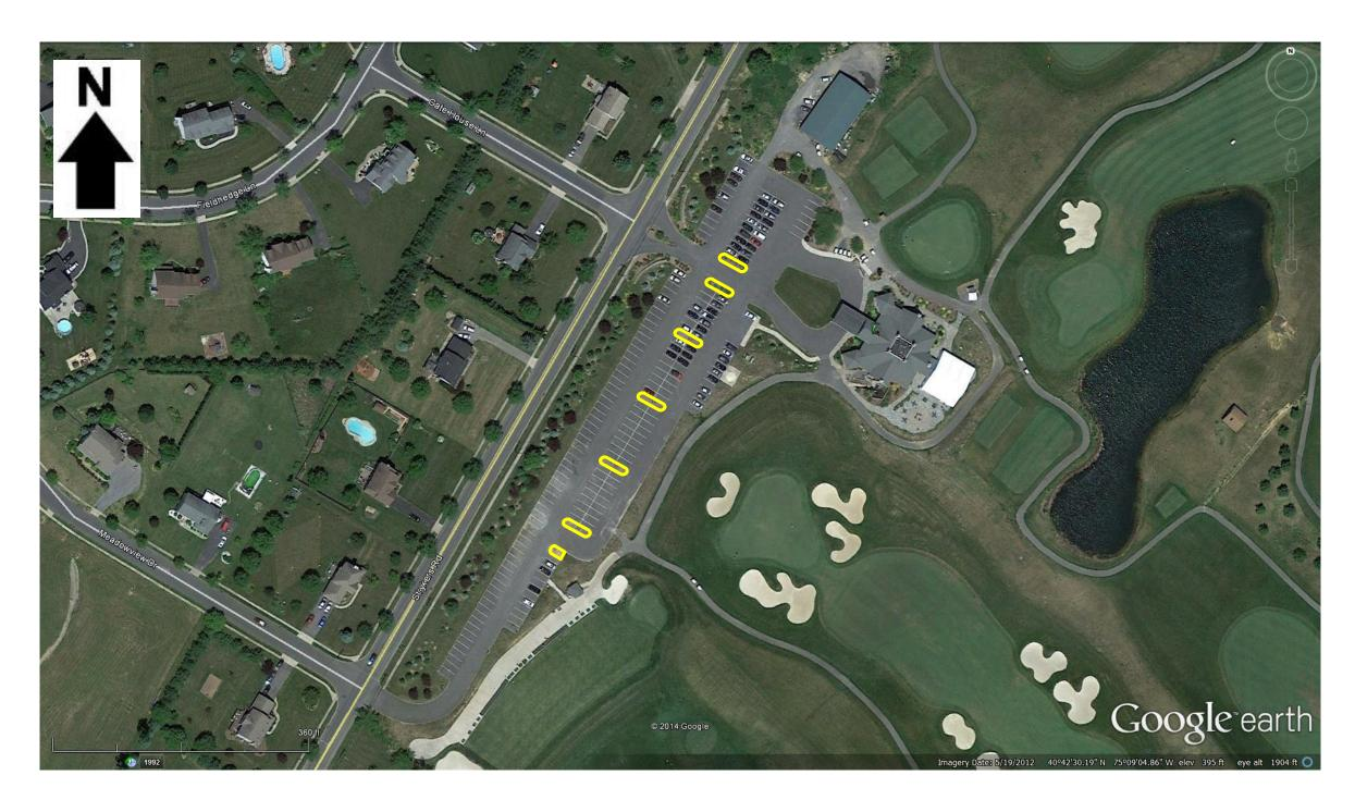
TREE FILTER BOX: The islands that are currently located in the parking lot could be converted to tree filter boxes. These tree boxes could capture, treat, and infiltrate runoff from the parking lot. Any excess runoff would be conveyed to the existing catch basins through an overflow bypass system. The tree boxes could reduce sediment and nutrient loading to the local waterway while accentuating the property's beautiful landscaping.
