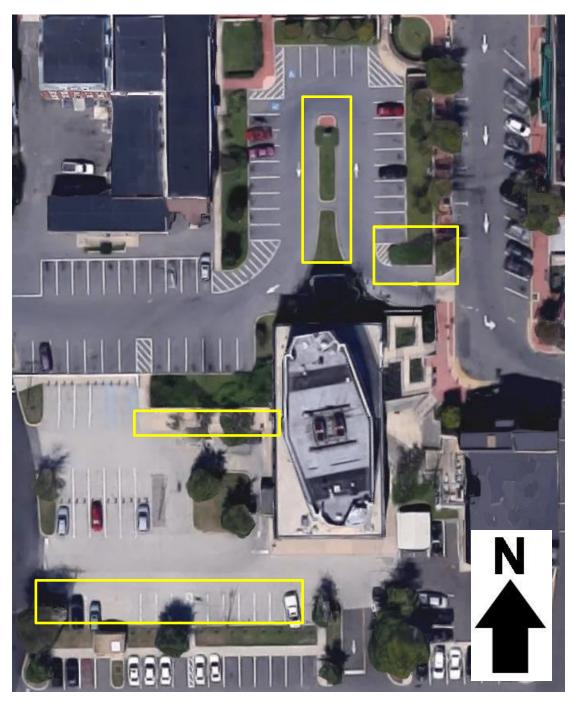
BIORETENTION SYSTEMS: Rain gardens can be used to reduce sediment and nutrient loading to the local waterway and increase groundwater recharge. This site has multiple areas where downspouts can be disconnected and rain gardens installed in the north parking lot area. Curb cuts can be made to allow stormwater to enter the bioretention systems from the street and parking lot.
