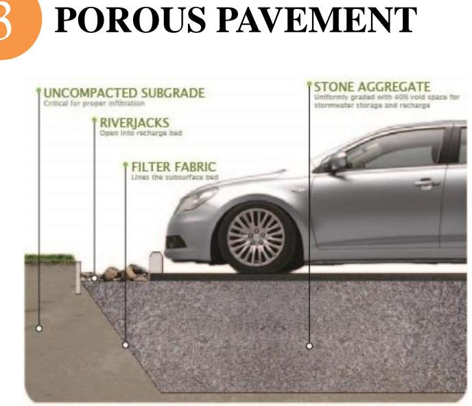
PERMEABLE PAVEMENT DIAGRAM
