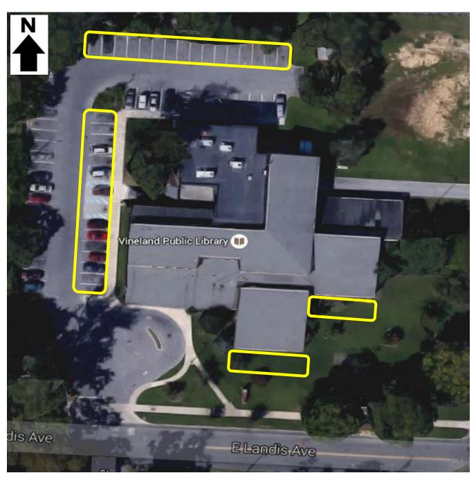
**BIORETENTION SYSTEM:** Bioretention systems could be installed adjacent to the library. The bioretention systems would reduce sediment and nutrient loading to the local waterway and increase groundwater recharge.
