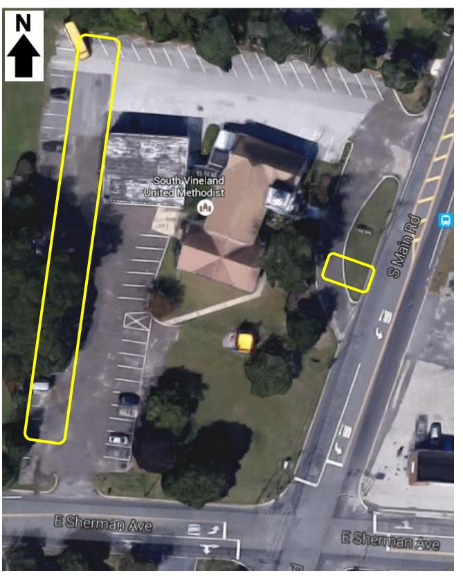
**DOWNSPOUT PLANTER BOX:** A downspout planter box can be installed on the eastern side of the church. This is a wooden box with plants installed at the base of a downspout that can provide an opportunity to beneficially reuse rooftop runoff.
