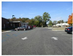
Installing rain gardens adjacent to the building and parking lot can capture, treat, and infiltrate runoff. A preliminary soil assessment suggests that the soils have suitable drainage characteristics for green infrastructure.
