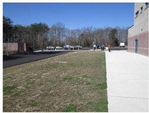
Installing a bioswale adjacent to the sidewalk can capture, treat, and infiltrate stormwater runoff. Rainwater can be harvested by installing cisterns in the courtyard of the building to capture roof runoff. Harvested rainwater can be used for watering plants. A preliminary soil assessment suggests that the soils have suitable drainage characteristics for green infrastructure.
