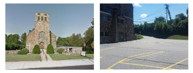
Stormwater is currently directed to the creek to the north that is downhill from the site. Parking spots on the north side of the parking lot can be replaced with porous asphalt to capture and infiltrate stormwater. A preliminary soil assessment suggests that more soil testing would be required before determining the soil's suitability for green infrastructure.
