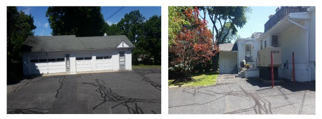
Stormwater is currently directed to the field behind the funeral home. Parking spots on the northeast corner of the parking lot can be replaced with porous asphalt to capture and infiltrate stormwater. A rain garden adjacent to the parking lot on the west edge can capture, treat, and infiltrate runoff from the roof and parking lot. A preliminary soil assessment suggests that the soils have suitable drainage characteristics for green infrastructure.
