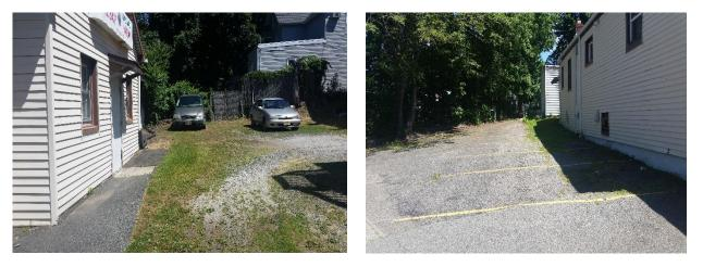
Stormwater is currently directed to an existing detention basin. Parking spots on the western side of the building can be replaced with porous asphalt to capture and infiltrate stormwater. A preliminary soil assessment suggests that the soils have suitable drainage characteristics for green infrastructure.
