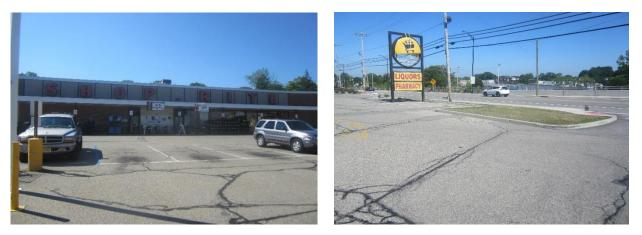
Stormwater is currently directed to an existing detention basin. Parking spots in the center of the parking lot to the north as well as the row of spots on the northeast corner can be replaced with porous asphalt to capture and infiltrate stormwater. A preliminary soil assessment suggests that the soils have suitable drainage characteristics for green infrastructure.
