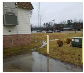
There are several locations around the municipal complex where rain gardens can be installed to capture runoff from rooftops and paved areas. An existing ponding area could be corrected by installing a bioswale that will convey water and allow stormwater to infiltrate. A preliminary soil assessment suggests that the soils have suitable drainage characteristics for green infrastructure.
