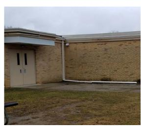
Rain gardens can be installed on both sides of the entrance to capture stormwater runoff from the rooftop. Pervious pavement can be installed in the parking spaces along the edge of the parking lot to capture additional stormwater runoff. A preliminary soil assessment suggests that more soil testing would be required before determining the soil's suitability for green infrastructure.
