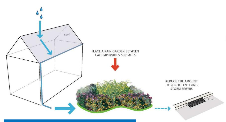
Rooftop runoff is now <u>"disconnected"</u> from flowing directly into the storm sewer system
