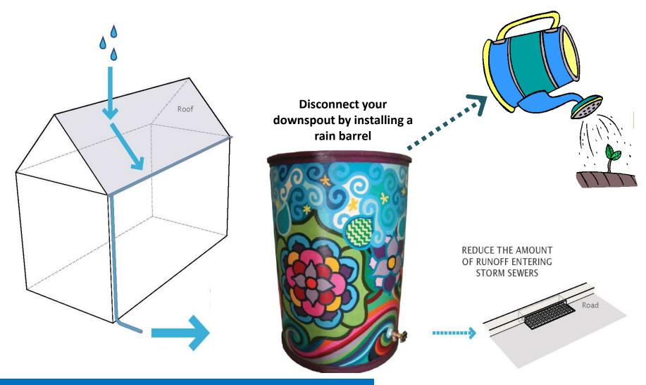
Impervious area is now <u>"disconnected"</u> from flowing directly into the storm sewer system
