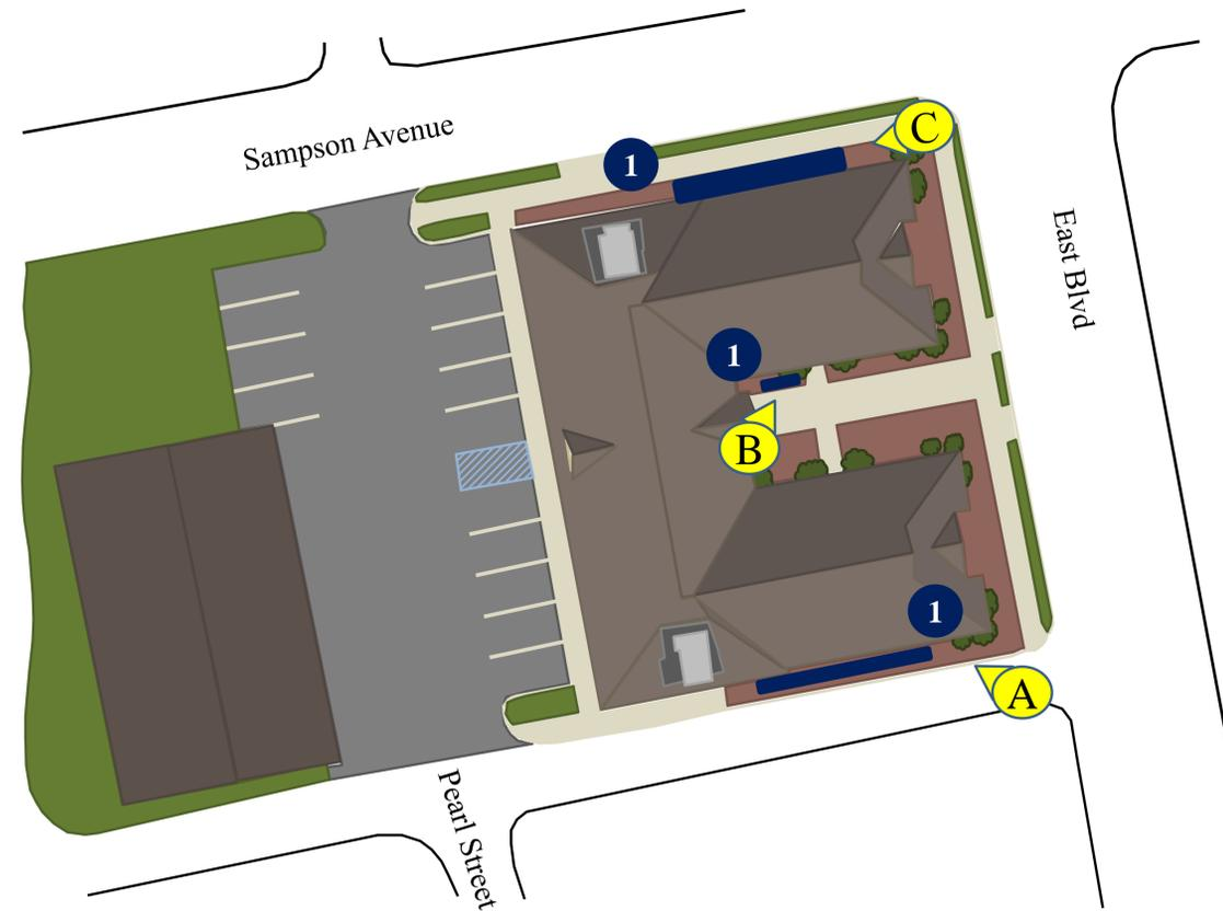
**1 DOWNSPOUT PLANTER BOX:** Downspout planter boxes can be installed by disconnecting and redirecting the connected downspouts into the planter boxes to allow stormwater runoff from the roof to flow into them. Planter boxes can intercept, treat, and filter a portion of the rooftop runoff.
