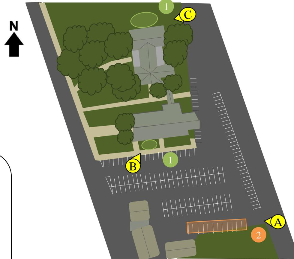
**1 BIORETENTION SYSTEMS:** Rain gardens can be used to reduce sediment and nutrient loading to the local waterway and increase groundwater recharge. This site has two areas that would be good locations for rain gardens. The proposed rain gardens sites are on the north side of the church and the south side of the school.
