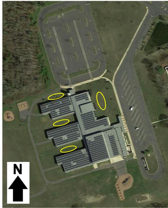
**1 BIORETENTION SYSTEMS:** Rain gardens can be used to reduce sediment and nutrient loading to the local waterway and increase groundwater recharge. This site has four locations: one near the entrance to the northeast and three others along the west side. All of these rain gardens could capture runoff from downspouts, many of which would be disconnected.
